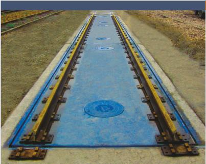
This weighing system is usually used for testing newly serviced or new wagons or locomotives to measure the load weight on each wheel. This is to make sure that total weight of wagon or locomotive is distributed evenly on all the axles. The only designer of Tear Load Press & Level Calibration in Asia.
